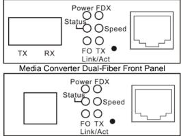
Media Converter Single-Fiber & SFP Front Panel
